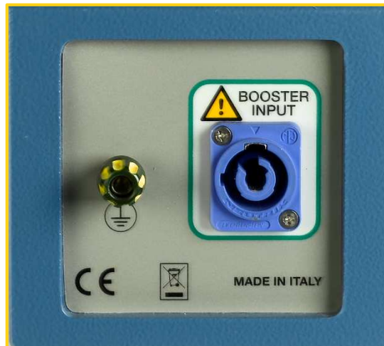
Figure 30 - Power supply on the side
