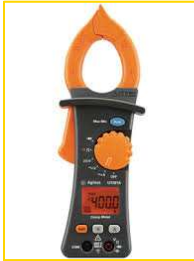
Figure 27 – Current Clamp Meter
