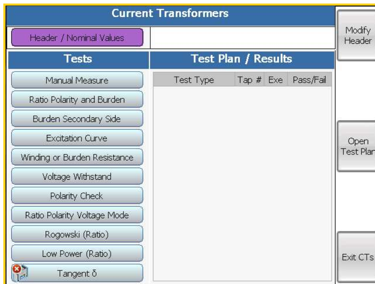
Figure 11 - "Current Transformers" test page (Conventional Type)
