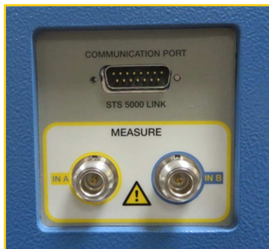
Figure 31 - IN-A (UST-A) and IN-B (UST-B) measurements on the side
