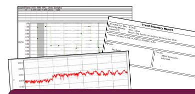
Reports can be displayed on a PC and printed. Each report includes all test results in a tabular and graphic format, as well as operator and test site information. Comments typed by the operator will also be included.
