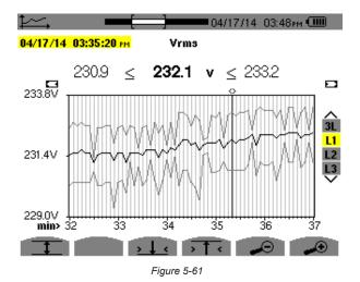
This graph differs slightly from the one shown in Figure 5-60 because, with the MIN-AVG-MAX mode, there is no loss of information.
