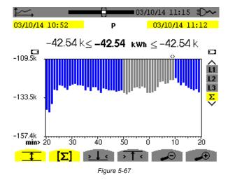
With the MIN-AVG-MAX mode activated, the display differs slightly from the previous one because there is no loss of information.
