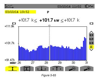
This graph (Figure 5-65) differs slightly from the previous one because, with the MIN-AVG-MAX mode, there is no loss of information.
