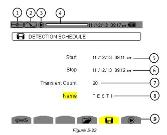
Item Function 1 Reminder of the mode used 2 Display of sub-mode used 3 Flashing Dicon: indicates that the search has been started 4 Memory indicator. Black area = used memory; White area = available memory 5 Transients search start time 6 Transients search end time 7 Number of transients 8 Name of transient Display a list of searches; Program a search; Start a search
