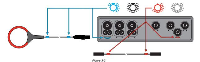
• Connect the measurement leads to the terminals of the instrument (see § 2.8).
