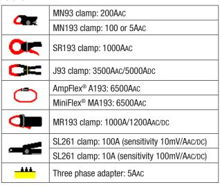
If an MN193 clamp, 5A range, or an Adapter is used, the current ratio setting is proposed automatically. The configuration is done as follows:
