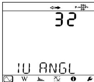
Phase angle between line current and phase voltage (3-phase 3-wire \Delta balanced)
