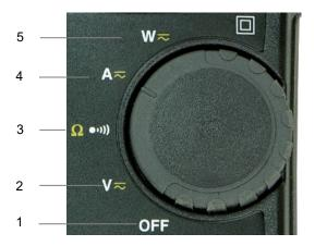
Figure 2: Function Rotary Switch
