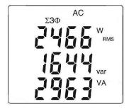
**NOTE:** 3-phase power on a balanced 4-wire network can also be measured by proceeding in the same way, or by proceeding as for the measurement on a single-phase network, then multiplying the value by three.
