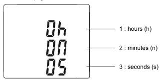
The duration of the metering uses the following format: XXXh (for hours) XXm (for minutes) XXs (for seconds).
