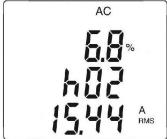
2. The Hz button can be pressed to display the frequency of the order of harmonic concerned.
