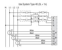
Diagram 5: Diagram 6: 3-Phase 4-Wire Wye Direct Voltage Input Connection 3-Phase 4-Wire Wye Connection 3 CT 3 PT
