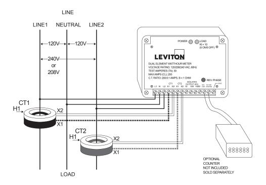
Leviton provides solid core CTs to achieve revenue grade accuracy. Our 100A and 200A color coded CTs assist with correct installation by indicating phase monitored.
