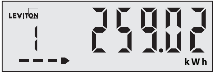
Figure 7 - LCD Appearance in Proper Operation (Example)
