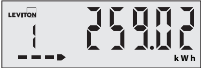
Figure 7 - LCD Appearance in Proper Operation (Example)
