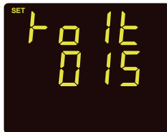
Fig 3-30 RO1 Alarm Delay Setting
