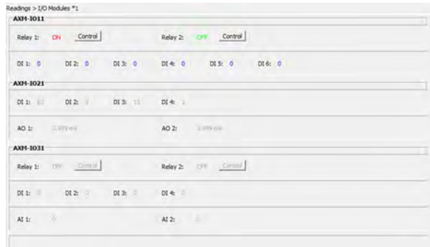
Figure 5-32 Relay Output Readings from Acuvim Software
