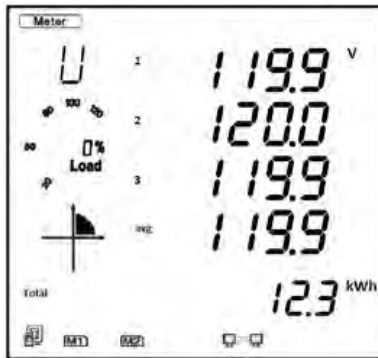
Figure 3-3 - Three-Phase Voltage Page
