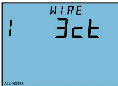
Fig.3-41 Current input wiring setting
