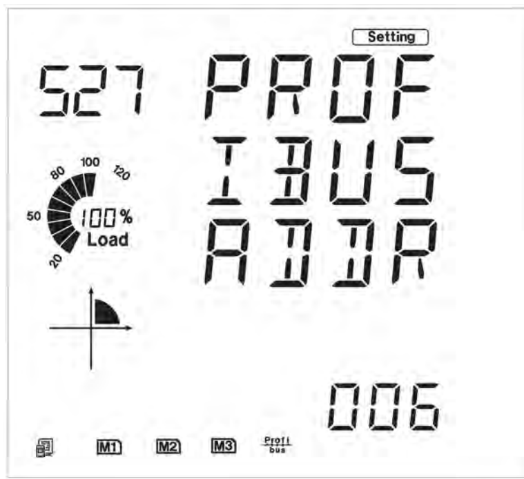
Fig 5-55 Address setting of PROFIBUS module
