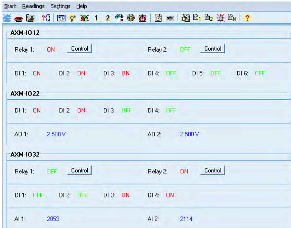
Fig 5-12 functions of IO modules
