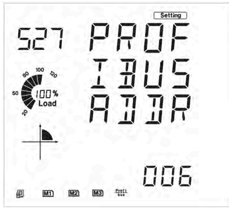
Fig 5-55 Address setting of PROFIBUS module
