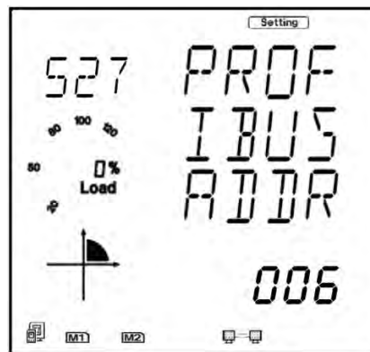
Figure 5-50 AXM-PROFI address setting on meter display
