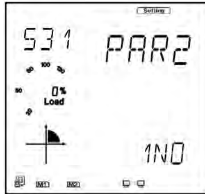
Figure 5-54 Parity setting for the AXM-RS485 module
