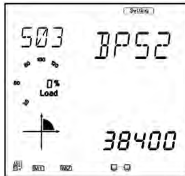
Figure 5-53 Baud Rate setting for the AXM-RS485 module
