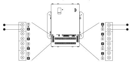
2. Connect 2-wire 100-277 VAC power to the control power terminals. Observe polarity. Connect voltage lines to the voltage taps. Equip voltage lines with fuses and disconnects as required.
