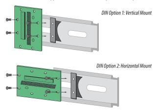
B. SNAPTRACK: Secure the SNAPTRACK to the mounting surface. Click the adapter board into place.
