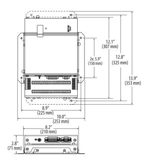
Note: The dotted lines indicate dimensions if the two brackets are placed for horizontal mounting. At the factory, the brackets are placed for vertical mounting. See Installation section for more information.
