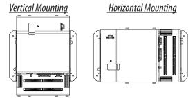
2. Install the E31E in the panel (hardware not provided). A grounding connection is located on the housing (see below). Use this stud to ground the device when it is mounted on a nonconductive surface.
