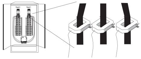
Note: The E31E measures and reports the phase angle of each voltage input and each CT (when there is active current through the primary of that CT). Use the E3x Configuration Tool to view the phase angles of active circuits to help verify that those circuits are connected to and mapped to the proper voltage phases. See the E3x Commissioning Guide for instructions on how to download and operate the tool from a PC.
