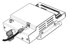
7. Once configured, disconnect the local PC. If desired (and the device is configured for operation on the network), connect the E31E directly to the network for ongoing access to the GUI even if primarily using a serial protocol to access and control the
