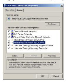
e. Select < Use the following IP Address >. Make note of the IP address that appears, then enter the static IP address (e.g. if the E31E Series is still set to its default address of 192.168.1.24, then change it to 192.168.1.100). Enter for the 255.255.255.0 subnet mask. Click OK.
