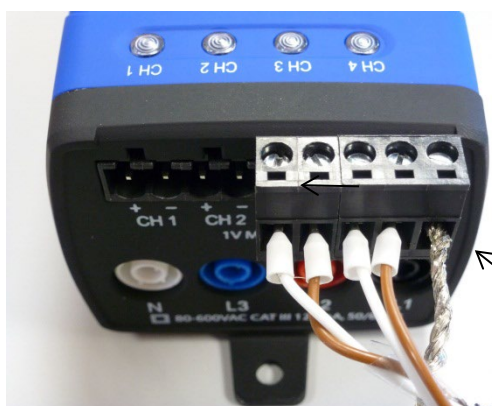
Connecting RōCoil CTs to an ELITEpro XC
