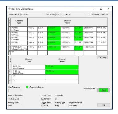
Once connected to an actual load, allow the logger to collect several minutes of data. Then review the collected data to ensure the readings make sense for your setup. Collected data can be saved as an .elog file on the hard drive.
