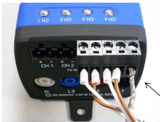
Connecting RōCoil CTs to an ELITEpro XC
