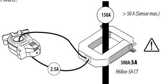
DANGER: 5A CTs can present hazardous voltages. Install CTs in accordance with manufacturer's instructions. Terminate the CT secondary before applying current.
