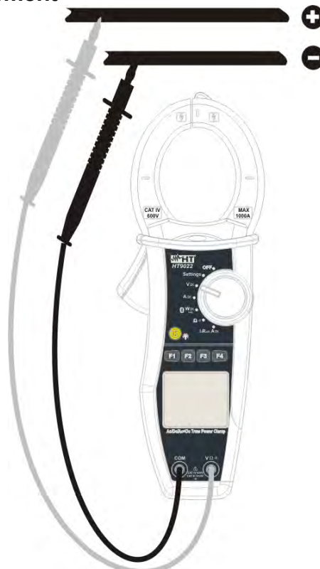
Fig. 5: DC voltage measurement
