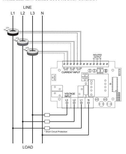
Leviton recommends solid core transformers (CTs) for revenue-grade accuracy. Our 100A and 200A color coded CTs assist with correct installation by indicating phase monitored. Split core CTs are also available upon request for applications where power cannot be interrupted during installation. Our 100-1, 200 Amp Split Core CTs offer +/-1.0% accuracy.
