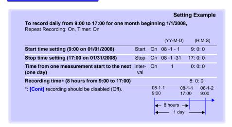
Measurement operation depends on the trigger, timer, repeat recording (On/Off), and recording time settings.
