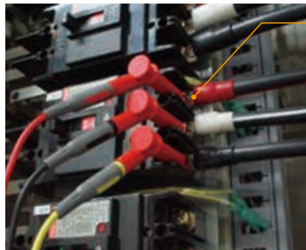
Magnetic design (diameter: 11 mm)
