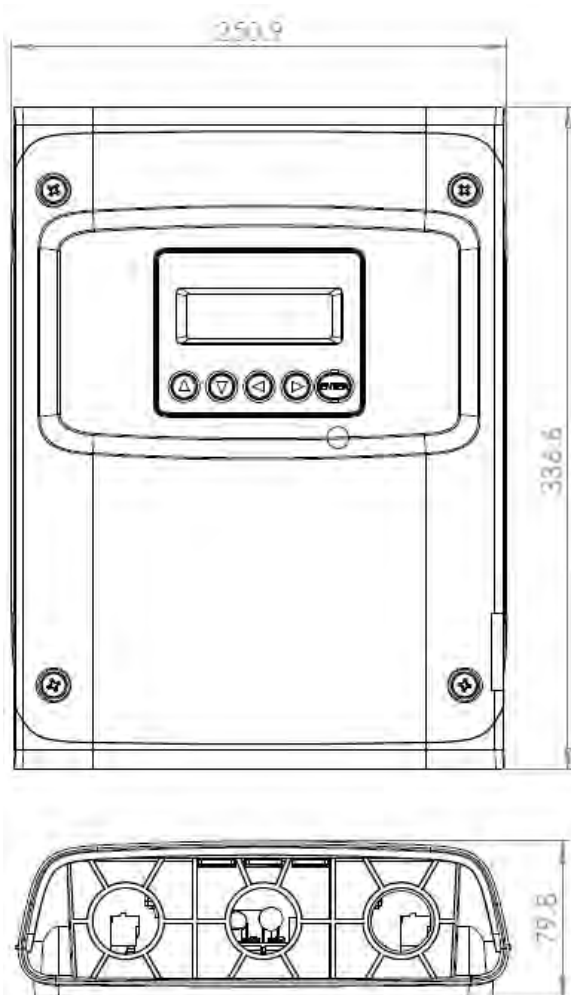
PS24HD/PS48HD Enclosure Dimensions
