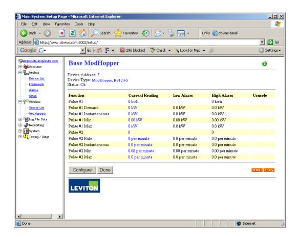
The EMH Hub will display will report all the data values present on the ModHopper. In addition, the instantaneous min/max rate values will be cleared after each logging interval. Click the Configure button to set up pulse input names, unit of measure and multipliers as needed.
