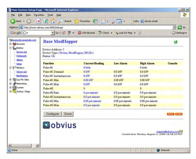
The AcquiSuite will display will report all the data values present on the ModHopper. In addition, the instantaneous min/max rate values will be cleared after each logging interval. Click the Configure button to set up pulse input names, unit of measure and multipliers as needed.
